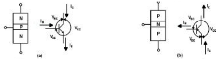
Figura 3: Transistor bipolar : (a) NPN (b) PNP
