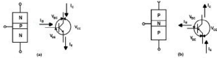
Figura 3: Transistor bipolar : (a) NPN (b) PNP
